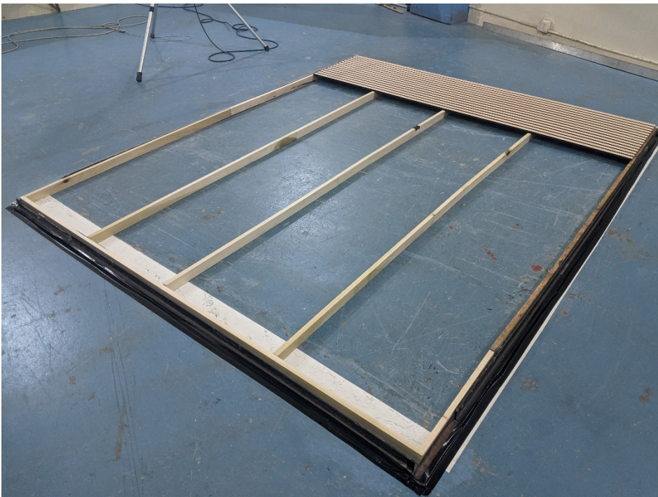
Figure 2 – Specimen partially installed over spaced furring strips
